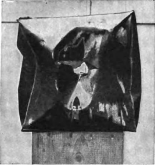
FIG. 6.—This tin was filled with water and struck by a brass slug, which passed clean through, compressing the water so that its recoil bulged out the tin into a barrel shape. The white lines indicate the corners of the box.
