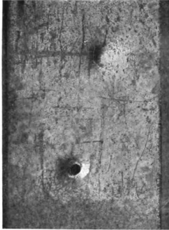
FIG. 1.—A rolled-iron plate, 1-8in. thick. The big dent at the top (½in. deep) was made by a wooden rod; the hole by a brass slug, which almost penetrated a board 2in. thick.
