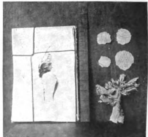
FIG. 9.—The magazines and projectile after discharge. Note the discs of paper of graduated size punched out of the magazines.
