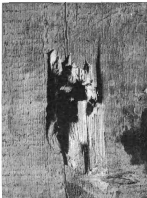
FIG. 11.—A 3-in. beam penetrated by shot.
