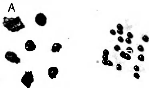
FIG. 10.—On the left are small lumps of lead, resulting from the fusing together of shot on striking an iron plate. The lump marked A is as heavy as twelve shot.
