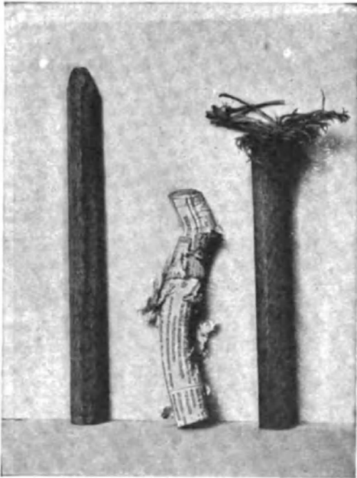
FIG. 2.—A wooden projectile before and after impact on a thick iron plate. Between them is a paper bullet, telescoped by an unsuccessful attack on the same plate. Before being fired it was somewhat longer than the stick on the left.
